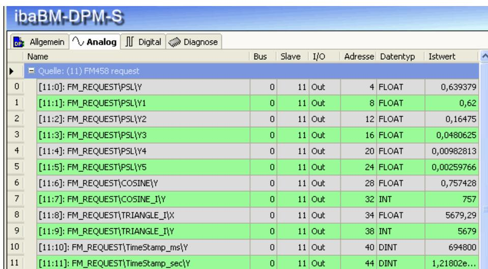
The screenshot shows the 'ibaBM-DPM-S' software interface. The 'Analog' tab is selected, displaying a table of measurement data. The table has columns for 'Name', 'Bus', 'Slave', 'I/O', 'Adresse', 'Datentyp', and 'Istwert'. The data is organized into a tree structure under 'Quelle: (11) FM458 request'.
