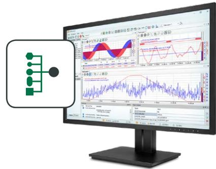
An ibaPDA system can be connected to TwinCAT controllers via EtherCAT or Ethernet communication. Which method is best depends on, amongst other things, how quickly the data needs to be acquired, whether scan-cycle-synchronous data transmission is required and which hardware is available. In addition, the Request method and the Xplorer interface offer the option of selecting signals using the symbolic identifiers via a symbol browser without any programming effort.
