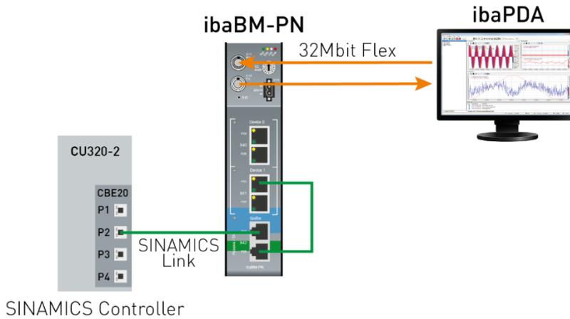
To enable data acquisition at the SINAMICS Link with only one controller, one of the two PROFINET devices can be switched to the SINAMICS emulation mode. The device can then no longer be used as a normal PROFINET device.
