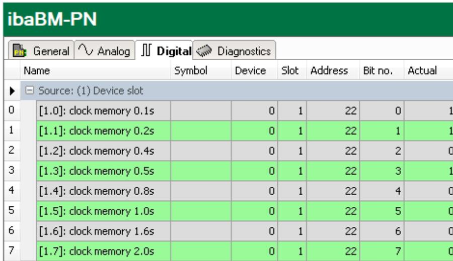
The screenshot shows the 'Digital' tab in the ibaBM-PN interface. It displays a table with the following columns: Name, Symbol, Device, Slot, Address, Bit no., and Actual. The table lists 8 digital signals, all from device 0 in slot 1, with addresses 22 and bit numbers 0 through 7. The 'Actual' column shows the current state of each bit.
