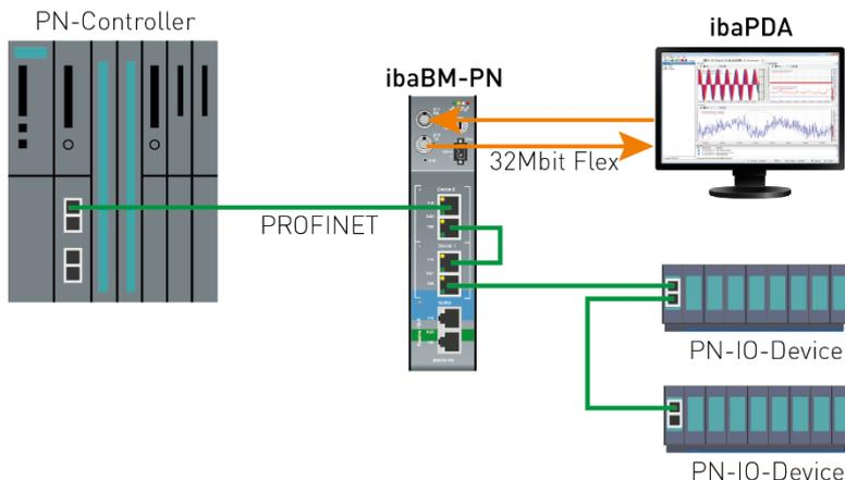
In the example above, both ibaBM-PN PROFINET devices are used by one PROFINET controller. For this purpose, both devices have to be entered via the GSDML file in the configuration of the PROFINET controller. The two PROFINET devices are connected with a patch cable.
