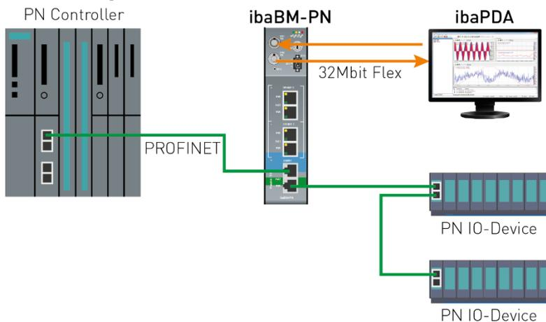
In the above example, the TAP interface is used for acquiring and analyzing the transferred data without interferences. It does not have to be integrated into the configuration of the PROFINET controller.
