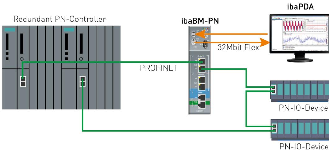
PROFINET system redundancy is distinguished into three configurations with the designations S2, R1 and R2. ibaBM-PN only supports "S2" configurations.
