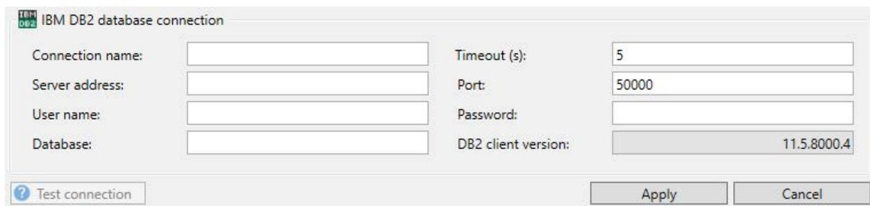
From the *Data source* drop-down list, select *Create new connection* and select the database provider.
