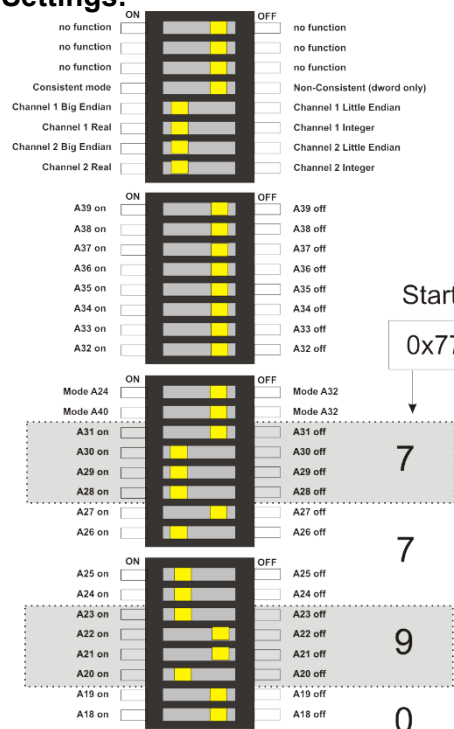
Figure 5 DIP switch, settings for ALSPA C80 HPC (one, respectively first ibaLink-VME card)
