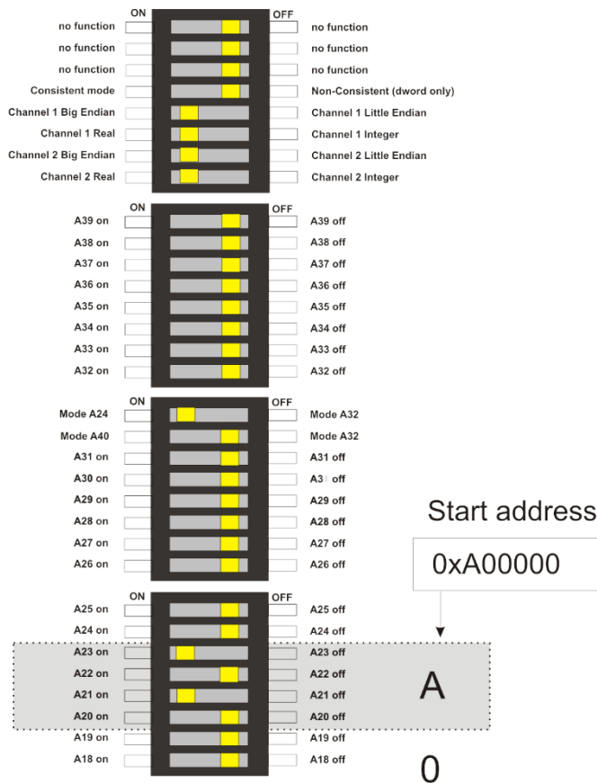
Figure 9 DIP switch, settings for GE 90/70 (one, respectively first ibaLink-VME card)
